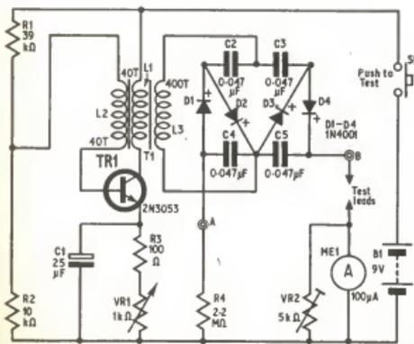
Fig. 1. Circuit diagram of the Megohmmeter
