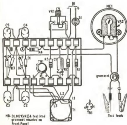
Fig. 2. Layout of the components on the tag-board and interconnections to the transformer, potentiometer, pushbutton and meter.
